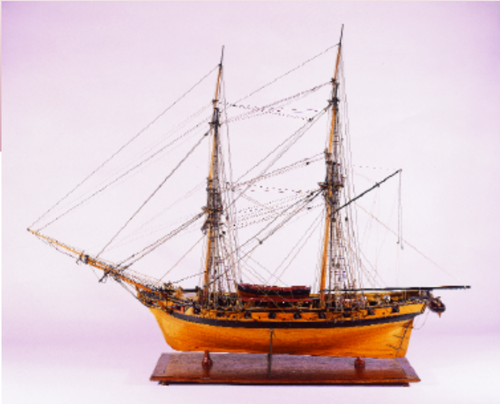
An English dockyard model of an 18-gun brig-of-war, period 1804, scale: 1/4" = 1'. Modelmaker(s) unknown. Dockyard models were most often used by navies to study a new design or method of construction. This example has a fully-fitted interior, indicating that it was also used to study crew accommodations and hold arrangement. Photo: Erik Ronnberg.
